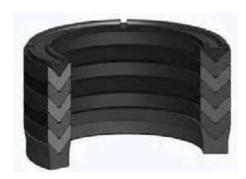
K04 is a seven piece single acting sealing set which consists of one reinforced cotton fabric backup ring, one thermoplastic header ring, three reinforced cotton fabric middle rings, and two elastomeric nitrile rubber middle rings.
