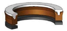
K151 is a three piece single acting chevron seal which consists of one thermoplastic header ring, one specially formulated reinforced cotton fabric with nitrile rubber sealing element and one PTFE back-up ring.
